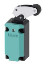
Position switch Plastic enclosure 40 mm according to EN 50041 Device connection 1 x (M20 x 1.5) 1 NO/1 NC quick action contacts Angular roller lever and plastic roller 22 mm
