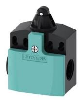
position switch plastic enclosure 50 mm device connection 2 x (M20 x 1.5) 1 NO/1 NC quick-action contacts roller plunger with plastic roller 10 mm
