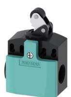
position switch plastic enclosure 50 mm, device connection 2 x (M20 x 1.5) 1 NO/1 NC quick action contacts, roller lever with plastic roller 13 mm
