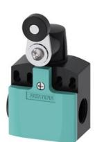
position switch plastic enclosure 50 mm, device connection 2 x (M20 x 1.5) 1 NO/1 NC quick action contacts, twist lever with plastic roller 19 mm
